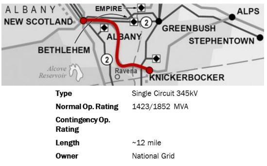
Figure 153: New Scotland-Knickerbocker Line Location and Parameters
