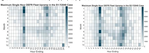
Figure 91: Maximum DEFR Fleet Up-Ramp (MW/hour) by Month and Hour: 2040 S1 and S2
