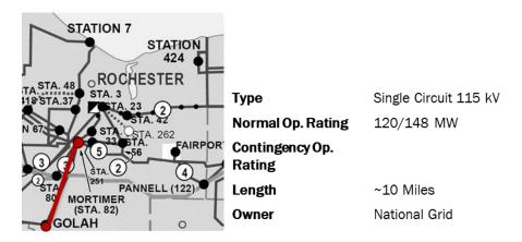
Congestion on this path is primarily due to UPV resources sited upstream of constraints that flow into load centers in zone B. The congestion increases on the line as more resources are added upstream of the constraint along the 115 kV corridor.
