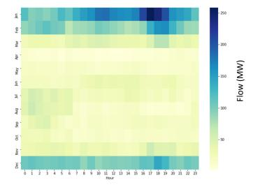
Figure 157: New Scotland-Knickerbocker Average Delta Flow
