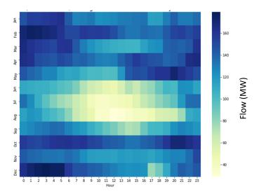
Relaxing the line limits on Barrett-Valley Stream increases the flow on the line significantly in the relaxed case compared to the Contract Case. The flow duration curves below shows a large delta in the later years compared to early years in the study period. Relaxing the limits on the line allows all of the renewable energy to export out of the interconnection point to serve load. The heatmap shows that the flow increases on almost all hours throughout the year.
