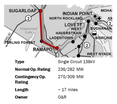
With upgrades associated with Segment B of AC Transmission, increased flow is observed on the 138 kV line from Sugarloaf to Ramapo. The projected congestion in the future years, starting in 2024 when AC transmission is modeled in service, is shown in the chart. Limiting contingencies include loss of higher kV circuits while securing this path.
