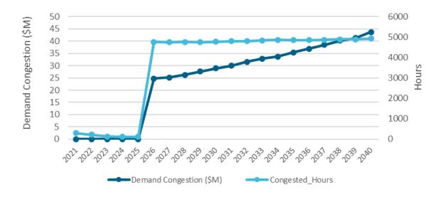
This line is congested very little prior to 2026 but the congestion increases significantly after offshore wind project is modeled in-service. The unit is injecting at a lower kV bus which is not designed to handle the amount of power produced by a large project. The violin plots below show a significant increase in line utilization starting in 2026 across all seasons.
