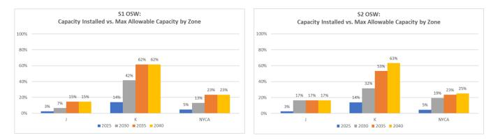
The progression of OSW capacity builds differed between S1 and S2; a higher amount of OSW capacity was built by 2030 in S2 comparatively, due to the lower limit on LBW capacity allowed by 2030, and the total amount of OSW capacity built by 2040 was slightly higher in S2 as compared to S1.
