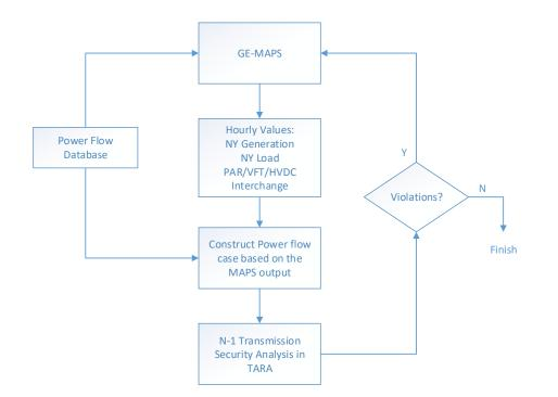
Figure 25 shows the flowchart for Roundtrip MAPS/TARA Analysis. This iterative analysis has three steps:
