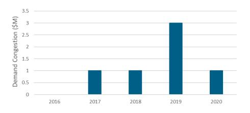
This path is located directly downstream of major generators in the New York System in and around the Oswego complex. Projected congestion on this path is directly related to generators operating upstream of the constraint and the contingency securing the flow on the line with lower limits.
