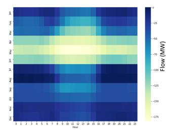
The relaxed case flows when compared to the Contract Case flows for the path below show that the flow on the path increases for about 20-30% of the year. Flow increase in the relaxed case occurs mostly during the summer peak period in the afternoon hours when loads are highest and fossil fuel generators are operating at their peak.
