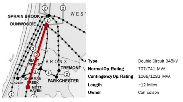
Figure 146: Dunwoodie-Motthaven 345 kV Line Location and Parameters
