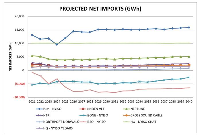
Figure 37 shows the projection of net imports on each interface for the Baseline Case. Net imports from Ontario decline with the retirement of the Pickering nuclear power plant in 2024 and 2025 and the refurbishment of the Darlington and Bruce nuclear power plants throughout the study period. Net imports from PJM increase in response to this refurbishment schedule. Across the other interfaces, net imports are largely flat through the study period.
