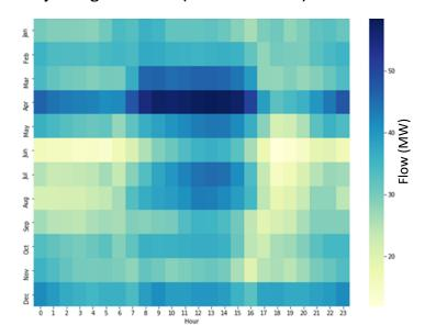
The relaxed case flows are marginally higher compared to the Contract Case flows. Flows on the line increases for about 20% of the year. Higher flows in the relaxed case usually occurs during the winter and spring period. Higher line flows are most likely due to nearby wind resources injecting additional energy on the line due to relieving congestion on the line.
