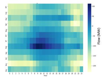
The relaxed case flows compared to the Contract Case shows that the flow does not have a significant increase when limits are removed from the lines in the relaxed case. Line flows increase for about 20% of the year in the relaxed case compared to the Contract Case. The heatmap shows that a large increase occurs in the peak load hours in the summer, and morning and evening hours in the winter season.
