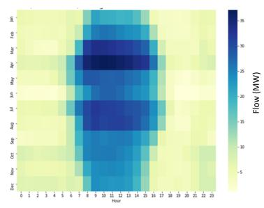
Relaxing the constraint by removing line limits along the path does not significantly change the flow on the line. The flow duration curve below shows the delta change in flow in the relaxed case as compared to the flow in the Contract Case. The relaxed case has higher flows in about 20% of the year in years after 2024. The heatmap shows that the increase in flow in the relaxed case occurs when UPV output is expected to be high and when more flow is expected flowing across the Central
