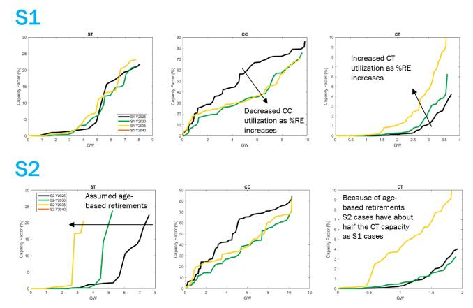
Figure 83: Fossil Fleet Cumulative Capacity Curve: Unit Level Capacity Factors
