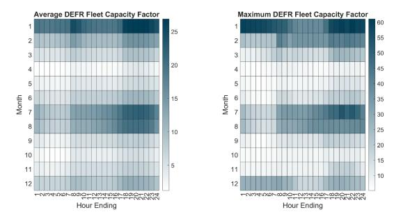
Figure 88: Average and Maximum DEFR Fleet Capacity Factors by Month and Hour: 2040 S1
